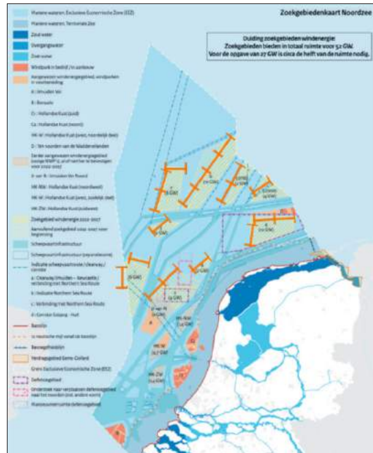
Figure 2 - Wind farm search areas by 2050, with assumed rows of wave devices. Each orange segment corresponds to 25 km.
